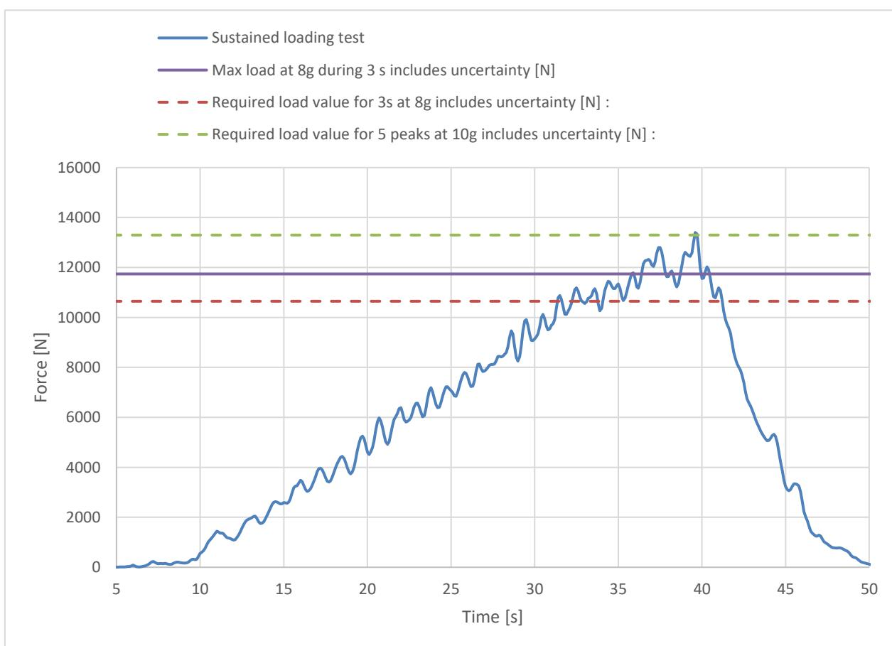
**Sustained loading test results <sup>(3)</sup>**Result: **POSITIVE**Calculated max load value with 3 sec or five peaks [kg]: **149.60**
